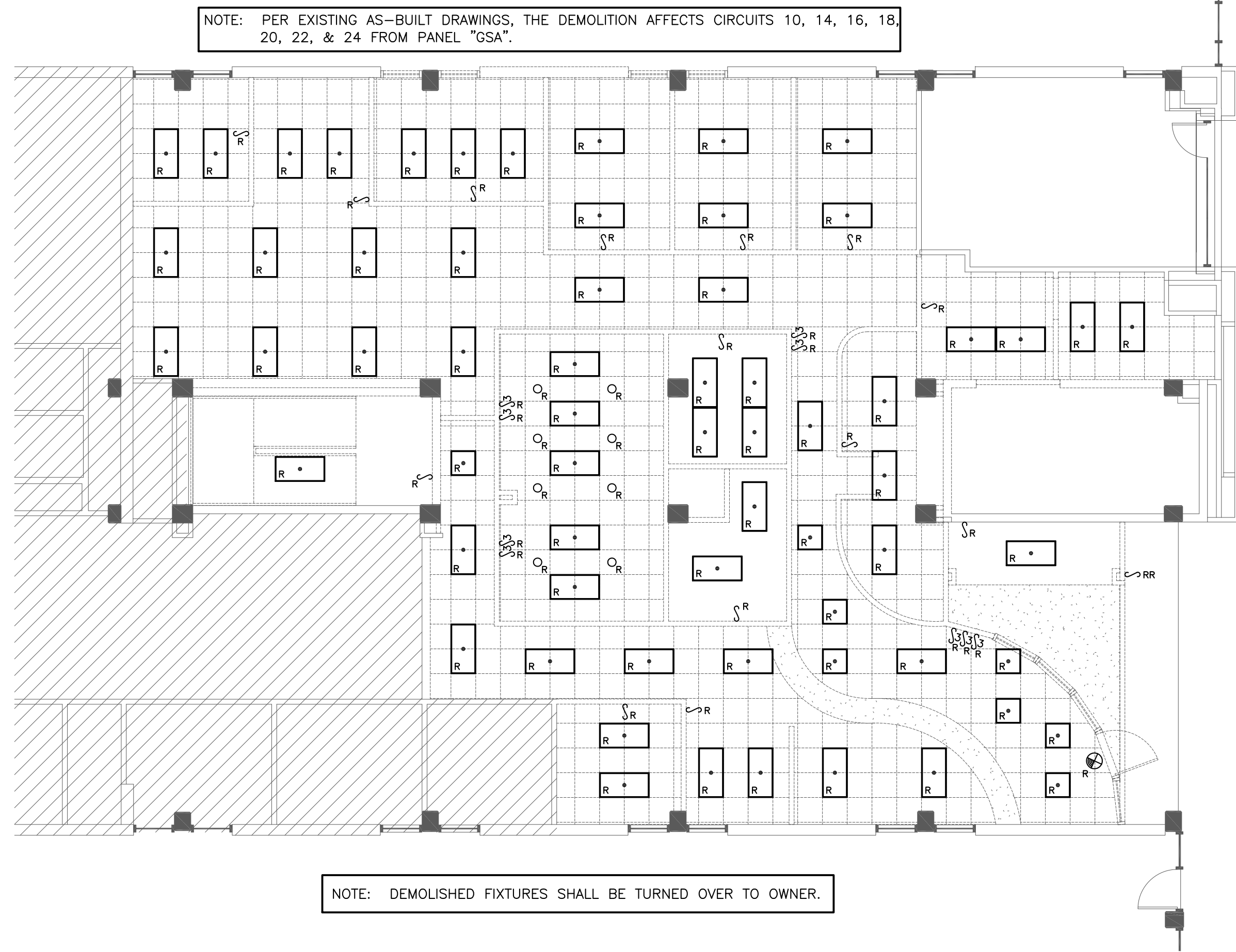
1 LIGHTING DEMOLITION PLAN SCALE: 1/8" = 1'-0"
